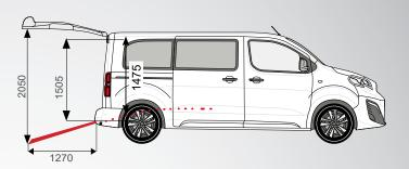
Entrance height 1505 mm | Useful internal height 1440 / 1475 mm | Lenght between WTORS 1303 mm | Width of wheelchair parking area 815 mm | Open ramp length 1270 mm | Open ramp width 765 mm
