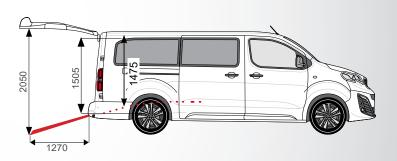
Entrance height 1505 mm | Useful internal height 1475 mm | Lenght between WTORS 1110 mm | Width of wheelchair parking area 815 mm | Open ramp length 1270 mm | Open ramp width 765 mm
