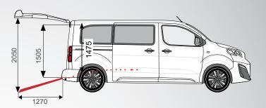
Entrance height 1505 mm | Useful internal height 1440 / 1475 mm |Lenght between WTORS 1303 mm | Width of wheelchair parking area 815 mm | Open ramp length 1270 mm | Open ramp width 765 mm \* configuration with optional swivel seats in 3rd row
