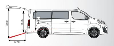
Entrance height 1505 mm | Useful internal height1475 mm | Lenght between WTORS 1110 mm | Length of wheelchair parking area 815 mm | Open ramp length 1270 mm | Open ramp width 765 mm
