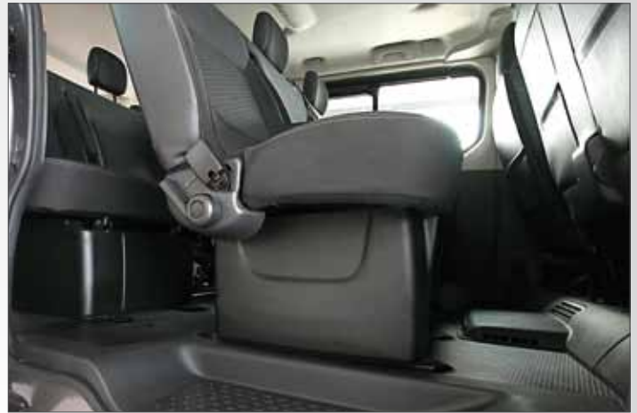
Side and front covers for the benches in second and third rows.
